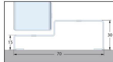
Optional 30mm open out threshold (must be specified if required)
